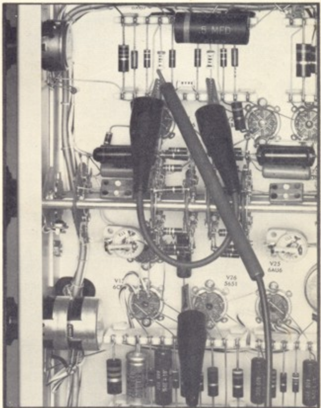
Fig. 6-8. Measuring the multivibrator screen voltage. Pins 6 of V1 and V2 are shorted together with a shorting strap. The meter leads are connected between the multivibrator screens and the A-150-volt supply. The M.V. SCREEN ADJ. control is adjusted for a meter reading of 80 volts.
